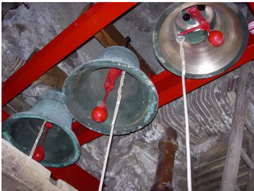
Rudry, nr Caerphilly, has a chime of 3 with trigger-action clappers (tenor 2 cwt 2qtr 6lb) (photo: Roger de Flaedenburg)
